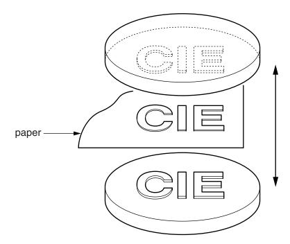
Design a hand-operated device that will allow the user to bring together the two discs shown above to leave an embossed shape on a single sheet of paper.
